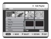
Press the ▲▼ buttons to select **Move**, then press the **OK** or **▶** button.
